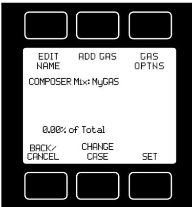
**GAS OPTNS** allows you to adjust the percentage of the constituents or delete a gas from the mix. Gas mixes cannot be adjusted after they have been saved.
