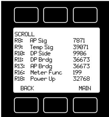
**DIAG TEST:** This diagnostic screen displays the current internal register values, which is useful for noting factory settings prior to making any changes. It is also helpful for troubleshooting with MATHESON customer service personnel.
