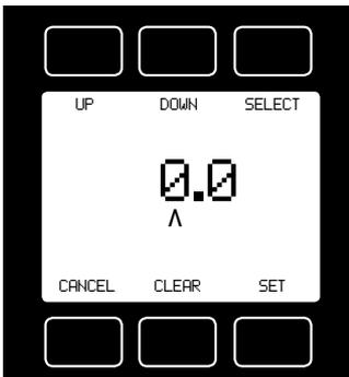
**Pressure Averaging and Flow Averaging** may be useful to make it easier to read and interpret rapidly fluctuating pressures and flows. Pressure and flow averaging can be adjusted between 1 (no averaging) and 256 (maximum averaging).
