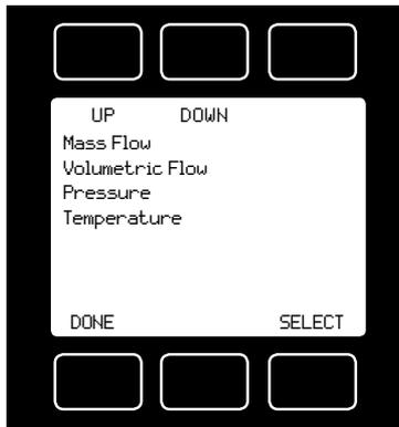
Press **DEVICE UNITS** to access menus of units of measure for each parameter. Scroll to the desired unit and press select. Once selected, you will see the message shown below. Verify that all connected devices expect the change. See pages 40 and 41 for a full list of available units.
