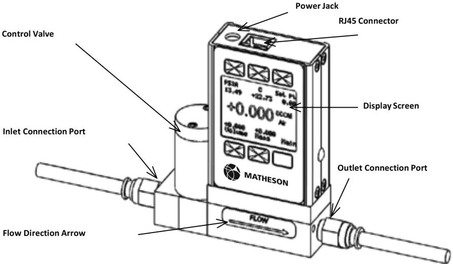
829 Mass Flow Controller shown with an upstream valve configuration and connection port fittings
