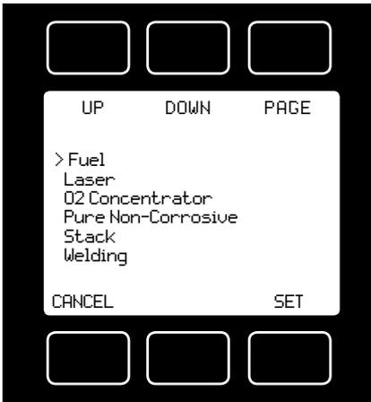
**Gas Select** allows you to set your device to up to 150 standard gases and mixes. You can also use **COMPOSER** to program and store up to 20 additional gas mixes.
