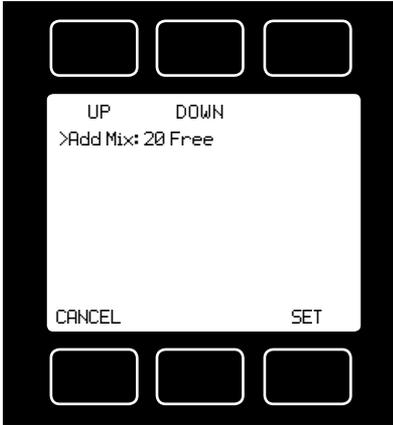
**COMPOSER** allows you to program and save up to 20 custom gas mixes containing 2 to 5 component gases found in the gas lists (pages 34-39). The minimum resolution is 0.01%.
