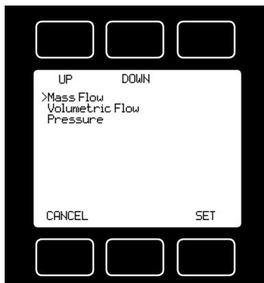
**LOOP VAR**—The selection of what variable to close the loop on is a feature unique to MATHESON mass flow controllers.
