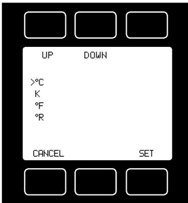
**Gas Temperature:** 829-Series flow controllers measure the incoming temperature of the gas flow. The temperature is displayed in degrees Celsius (°C). This parameter is moved to the primary display by pushing the button above **°C**.
